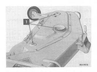
1 - Spindle bearings 44-inch and 50-inch mowers.
