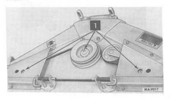
1 - Spindle bearings 38-inch mower.
