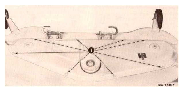
Nut, 5/16-inch and washers, 11/32 x 11/16 x .065-inch 7 required for 44-inch mowers 8 required for 50-inch mowers
