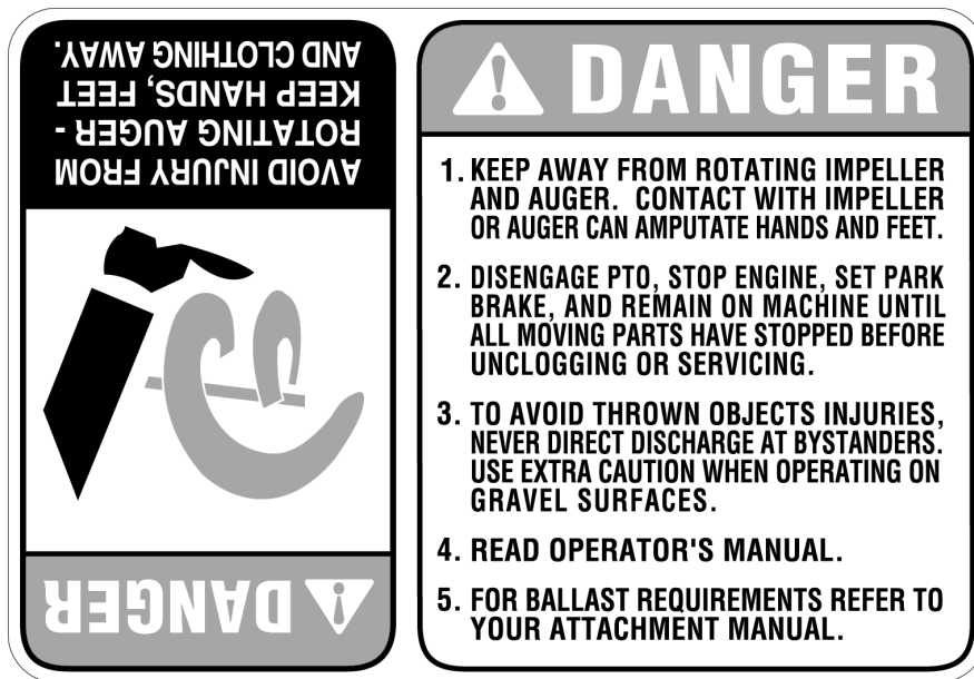
ON UPPER/REAR OF BLOWER HOUSING DANGER W/SCRIPT — FACING OPERATOR DANGER W/GRAPHIC — FACING FRONT OF SNOW THROWER
