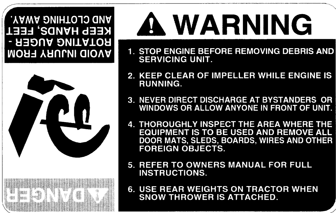
ON UPPER/REAR OF BLOWER HOUSING WARNING — FACING OPERATOR DANGER — FACING FRONT OF SNOW THROWER
